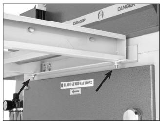
**Figure 12.** Roller table attached to mounting bracket.
